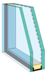
**Comfort glass** consists of tempered safety glass triple-coated with LoE, dual-sealed and injected with Argon gas. This quality glass provides excellent energy efficiency, thermal performance and protects against the sun's fade-causing UV rays.
