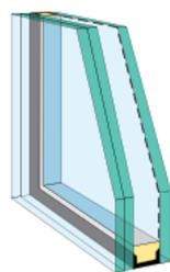
**ComfortPlus glass** consists of tempered safety glass triple-coated with LoE, dual-sealed and injected with Argon gas; Plus a laminated pane for added safety and protection from fade-causing UV rays.
