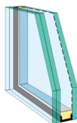
**EnergyPlus glass** consists of tempered safety glass over an interior pane of thicker laminated, LoE<sup>3</sup>, argon-gas filled glass designed for safety and energy efficiency providing three times more protection against solar heat gain.
